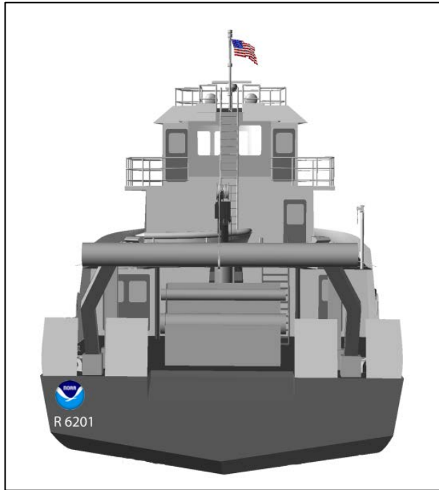
Figure 6: Example of NOAA emblem offset on transom due to obstruction by gear
