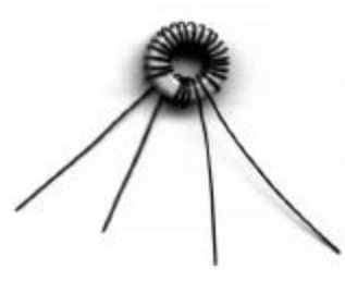
Completed T2 (T1 is the same except it has a 2 turn link winding, not 4 turns)
