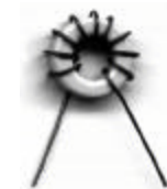
Completed L6 (L7 is the same, but with 1 turn less)
