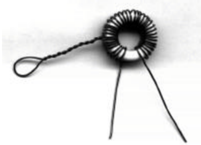
Completed L1 Toroid (Prior to cutting off the TAP loop)
