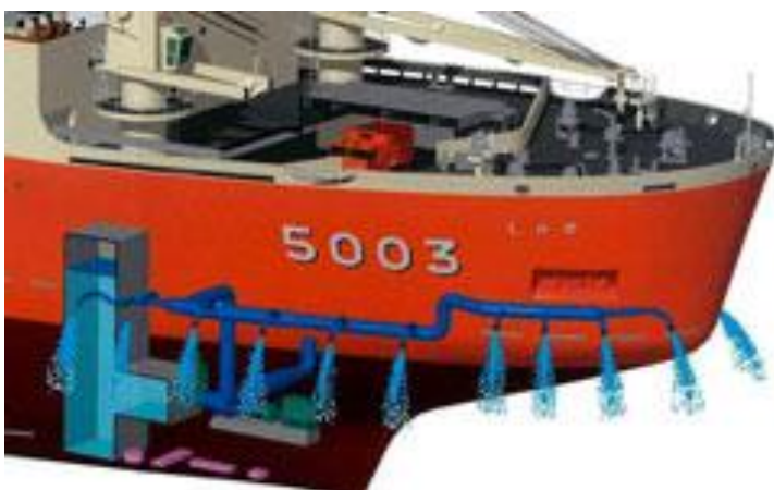
Figure 28: Hull Water Wash System
