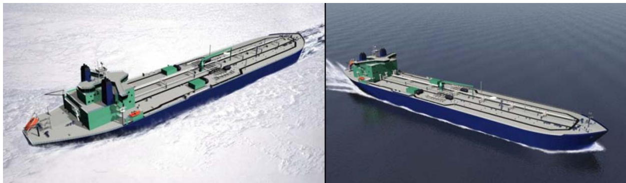
Figure 24: Double-acting Icebreakers: Astern on ice (left) and forward in open water (right)
