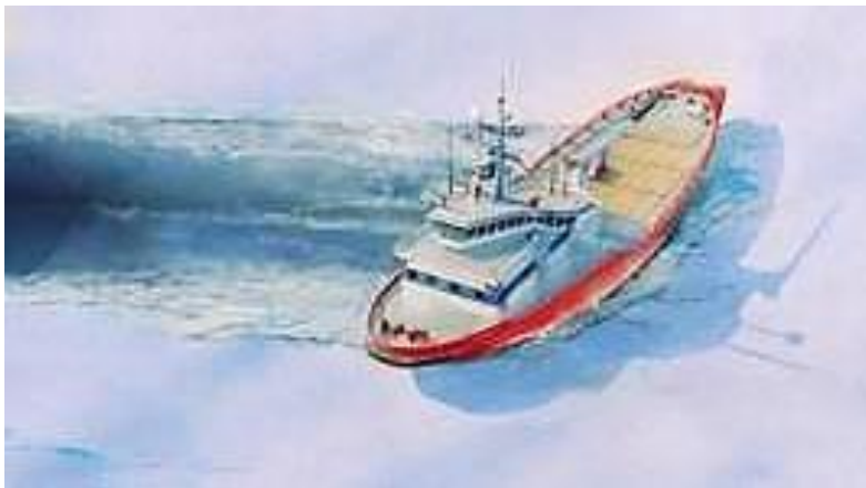
Figure 25: Sideways channel-clearing Icebreaker concept
