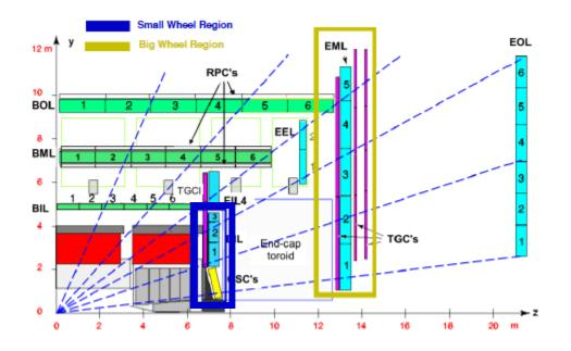
Current Small Wheel  $\rightarrow$  CSC, MDT (tracking), TGC (trigger) NSW  $\rightarrow$
