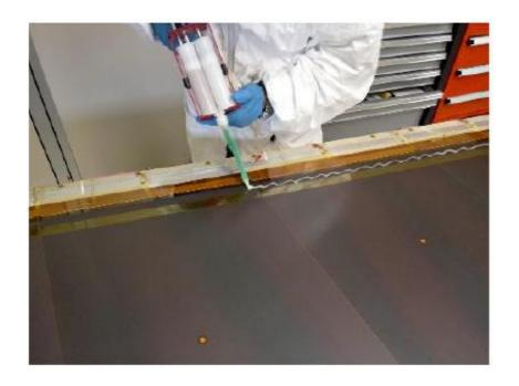
Width of passivated area such that R>0.8  $\mbox{M}\Omega$
