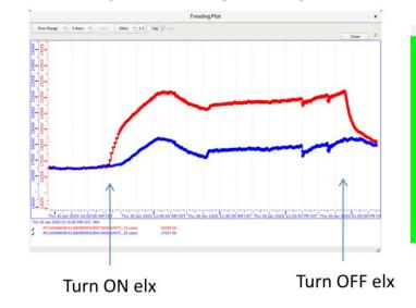
Water input and output temperatures
