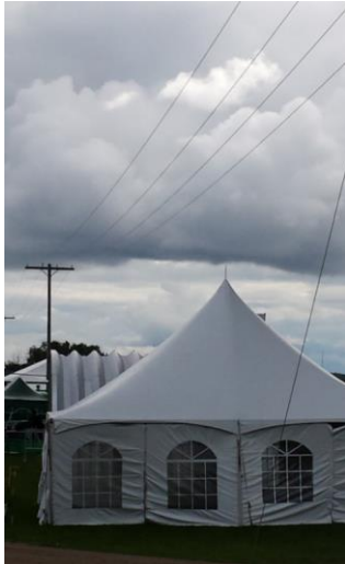
Fair tent set up under overhead powerlines
