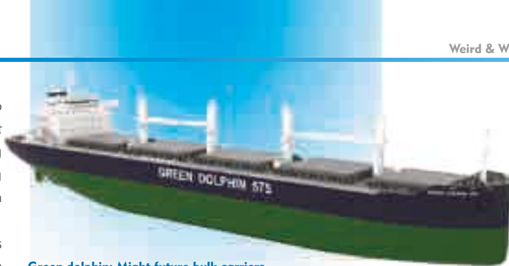
Green dolphin: Might future bulk carriers have straight stems for added wave resistance?
