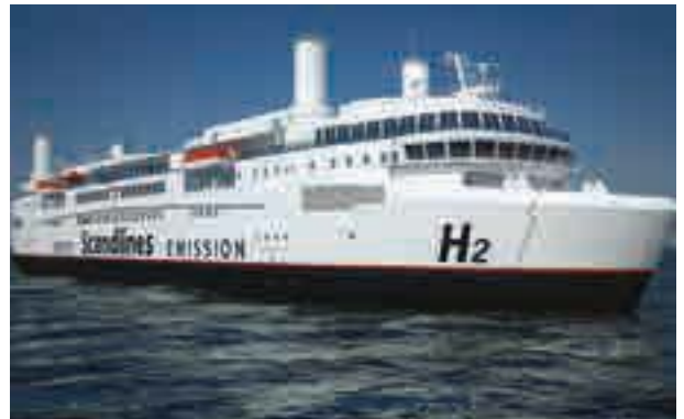
A zero-emission ferry project employs fuel cells, batteries and wind assistance through Flettner rotors
