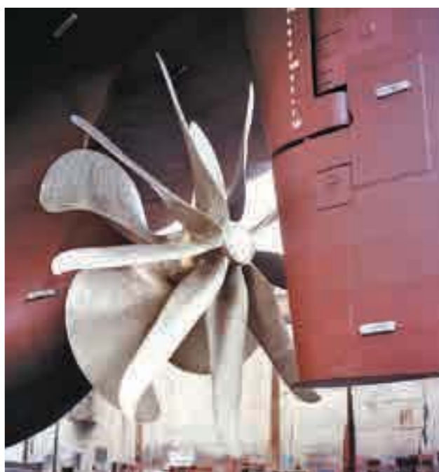
The propulsion improving Grim Vane Wheel, patented in the 1970s, could enjoy a renaissance
