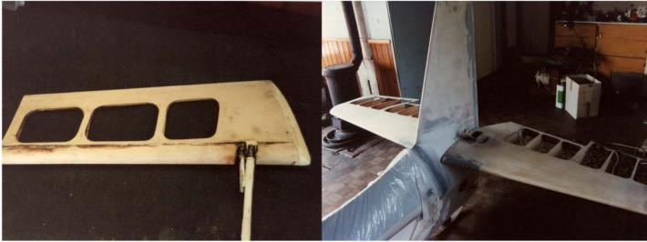
Left to Right. Port tailplane uncovered showing large lead balance weight in root of leading edge. One of the very large anti balance trim tabs. The uncovered tailplane half's in position.
