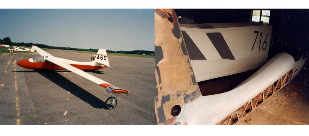
Left photo shows the 465 2 at Lasham shortly after it was purchased by Keith and myself. Note the transparent fairing in the centre section fairing. The glider was in very tatty condition. Right photo shows the fuselage stripped of fabric and filled ready for re covering.
