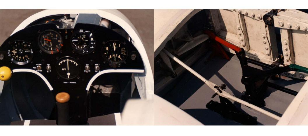
Left the instrument panel. Right the control connections . The red and green rods connect the ailerons the white ones are air brakes.
