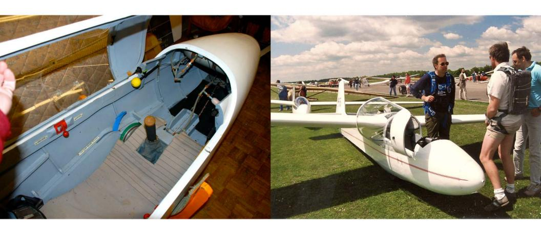
Left the inside of the cockpit with instruments removed. Note the green trim wheel, allegedly from a Wellington Bomber, very powerful trim on this glider. Blue air-brake lever, yellow cable release knob and red canopy catch. Right admirers at the launch point.
