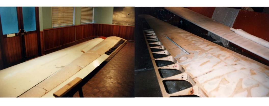
Left the wings in the process of being stripped of old fabric. Some re profiling under the leading edges was found, near the wing root. Right the white areas are micro balloon and epoxy resin filler to remove the rippling of the 1.5mm ply between the ribs.
