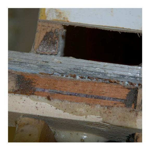
The reason for the gliders downfall. The thin white line between the metal and mahogany sections of the main spar is anaerobic inter-granular corrosion. This problem was discovered after a fatal accident to a 463. The corrosion on the 465 was worse than the glider which broke up. This is un economical to repair.
