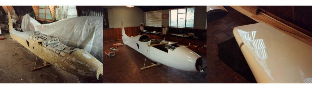
Left to right. Fuselage primed rubbed down and ready for a top coat. Sprayed and ready for re-assembly. Note the nose hook now fitted to avoid problems on aerotow. The rudder nice and shiny in its new paint.
