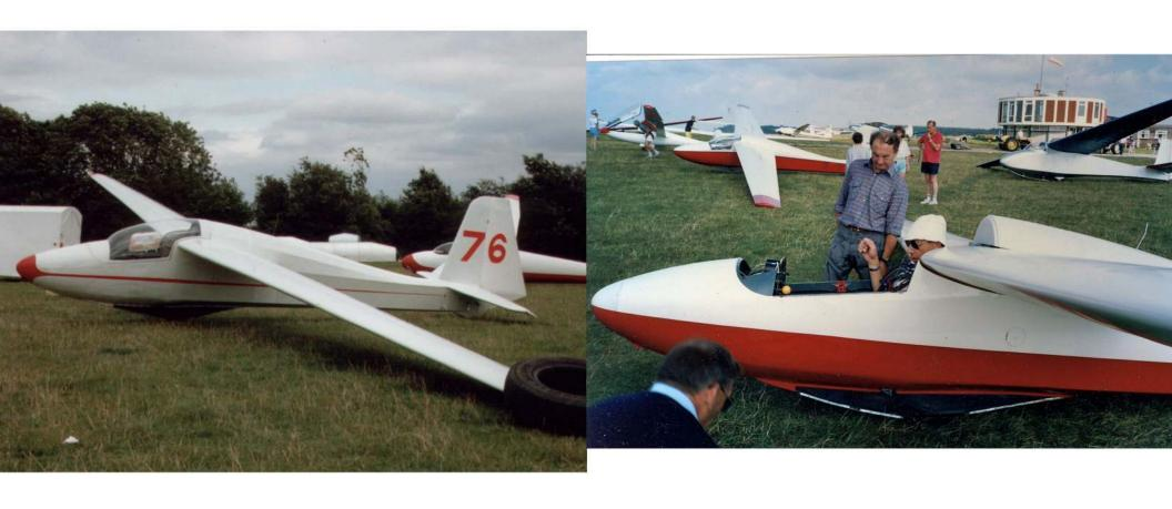
Left photo shows a 460. Note the skid, fabric covered rear fuselage separate elevator and lift off canopy. The right picture shows 2 463's with non structural fibreglass on the rear fuselage.
