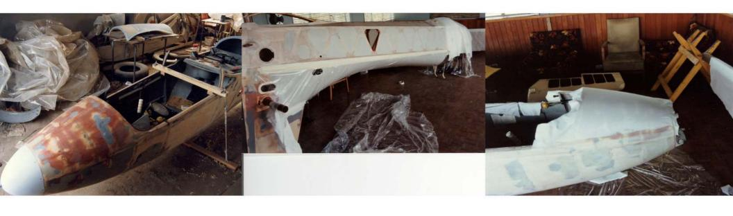
Left to right. Nose section filled and rubbed down. Centre the rear fuselage being re-covered. Right the nose covered but the fabric is not stretched and doped yet.
