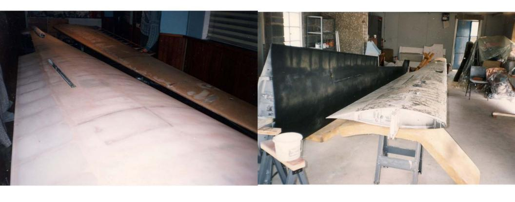
Left one wing covered and partly doped. Right the wings have been sprayed with silver UV protection then a primer surfacer. The primer is being rubbed down with fine wet and dry paper for a good finish. at least 90% of the work is in the preparation.
