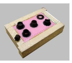
missing and four were damaged. I wanted to make a silicone rubber mold and cast new urethane resin replicas. Because of the damage to the original parts, it took some time to figure out how to prepare them to serve as
