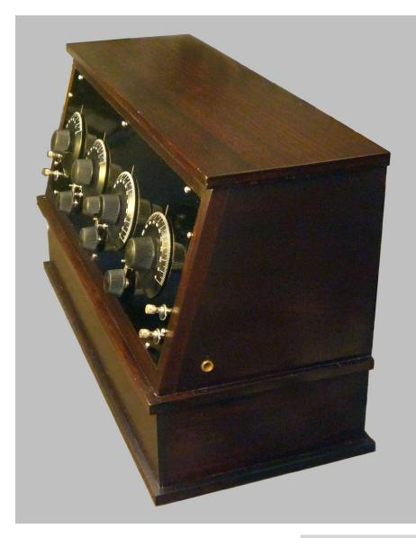
Note loudspeaker jack on side of cabinet. There is no mention of this feature in the literature. I presume it was a modification made by the assembler.
