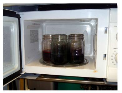
containing a length of washed plain cotton braiding on the turntable of my little shop microwave oven. After 5 to 7 minutes on high, I checked the solution temperature using my infrared thermometer; when it indicated I was at temperature, I found that setting the oven to a 'defrost' mode for one hour maintained the temperature pretty good.
