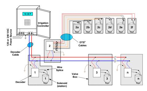
The following wiring diagram from a leading manufacturer of decoder systems shows the complexity of the wiring inside a valve box of a decoder installation. The average landscape maintenance contractor is not qualified to troubleshoot these kinds of systems.
