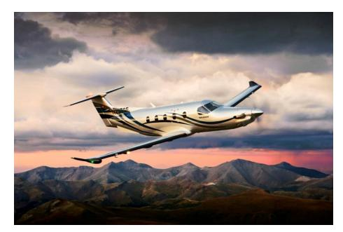
The Pilatus PC-12 NG is a high performance, single-engine turboprop, pressurized multi-mission aircraft certificated in the normal category.
