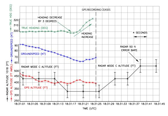
Figure 5 OK-OKD GPS and radar data
