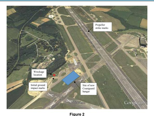
Accident site relative to the runway, looking back down Runway 30 from the direction of the Control Tower
