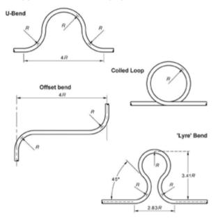
Expansion loops and offsets must be placed horizontally to avoid forming air locks at the top of the loops and to ensure proper circulation of the water. It is preferable to locate the bend or loop as close to the mid point of the straight run as possible.
