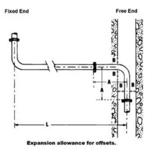
Fatigue cracks have sometimes occurred at bends in hot water lines where the tube passes from one structure to another, e.g. from a concrete floor up into a wall.
