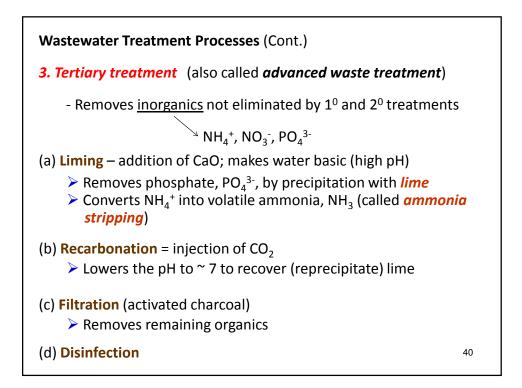
The third stage, known as *tertiary treatment*, varies depending on the community and the composition of the wastewater. Typically, the third stage will use chemicals to remove phosphorous and nitrogen from the water, but may also include filter beds and other types of treatment. Chlorine added to the water kills any remaining bacteria, and the water is discharged.
