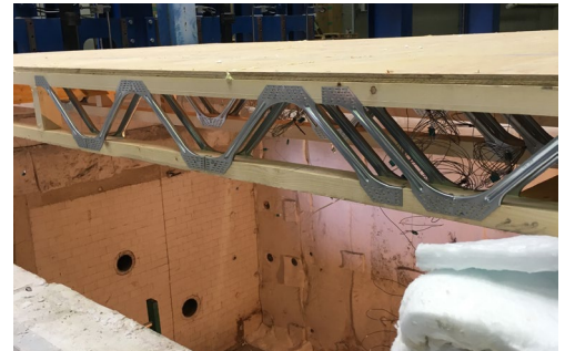
The following table describes Posi-Joist floors providing 30 minutes fire resistance to BS476-21
