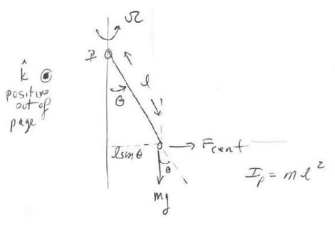
The torque about the pivot point is
