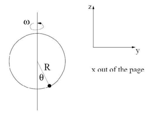
A bead of mass *m* slides without friction on a circular hoop of radius *R*. The angle  $\theta$  is defined so that when the bead is at the bottom of the hoop,  $\theta = 0$ . The hoop is spun about its vertical axis with angular velocity  $\omega$ . Gravity acts downward with acceleration *g*.
