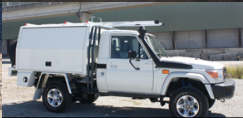
Toyota Landcruiser FleetPro II - with Roll Over Protection Bars (ROP's), Roof Bars & Ladder Holder, TradePro II Underbody Tool Box, Rear Platform & Spare Wheel Holders
