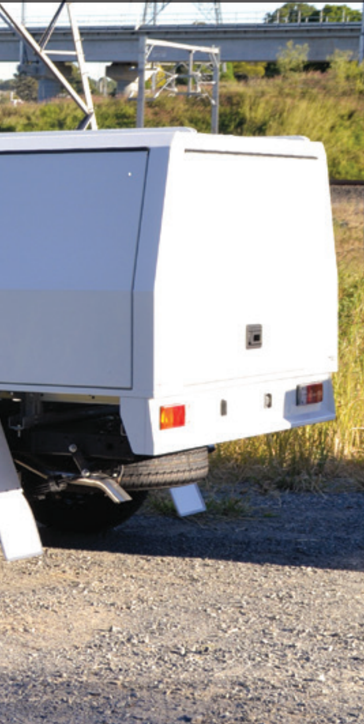
Toyota Hilux FleetPro II - with Rear Platform & Double Folding Spare Wheel Mount, Fold Down Step & Underbody Drawer Unit
