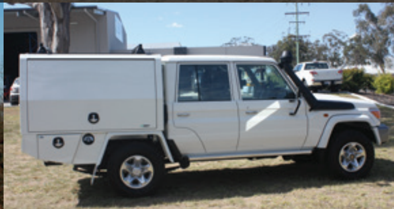
Toyota Landcruiser TradePro II - with Roof Bars, Upgraded Mudguards & Tail Light Channel, Fuel Filler Skirt Panel & Tapered Base Box
