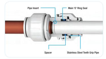
John Guest Twist and Lock® Fittings have a collet with stainless steel teeth that grip the pipe when fully inserted, and an O-ring to provide a permanent leak-proof seal. The additional benefit of the Twist and Lock fitting is that a twist of the screw-cap gives greater compression on the O-ring seal and locks the pipe in place for greater security.
