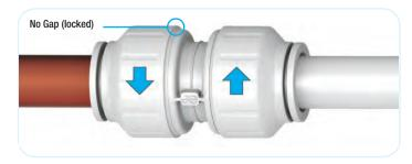
Twist the screw-cap until it touches the body flange. This locks the pipe into position and increases the o-ring seal around the pipe.
