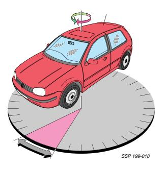
When the vehicle changes its direction of travel, it rotates about its vertical axis.
