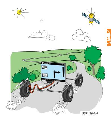
Vehicle navigation is the overall result of the interplay between satellite navigation and deadreckoning navigation.
