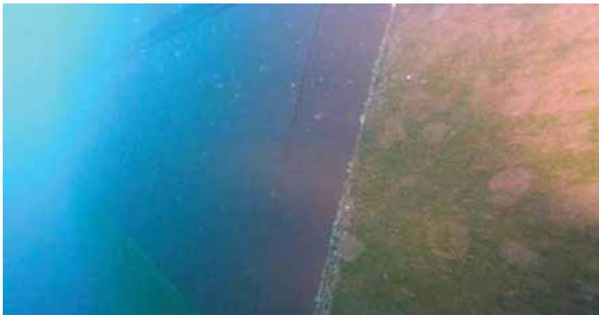
Figure 3: Silicone hydrogel test patch (left) observed completely free from fouling. Algae and slime observed on self-polishing A/F.
