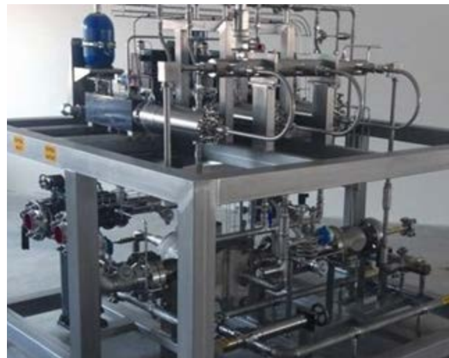
MAN Diesel & Turbo's prototype gas fuel pump and vapouriser unit (credit: MAN Diesel & Turbo)
