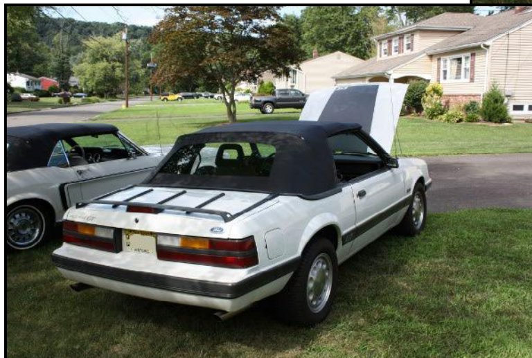
The third brake light in the luggage rack in a Convertible only
