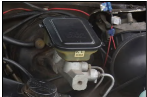
Dual-circuit master cylinder, separate reservoir, plastic cap
