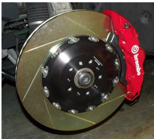
Disc brake system: disc (in gold), caliper (in red), pads (in caliper)
