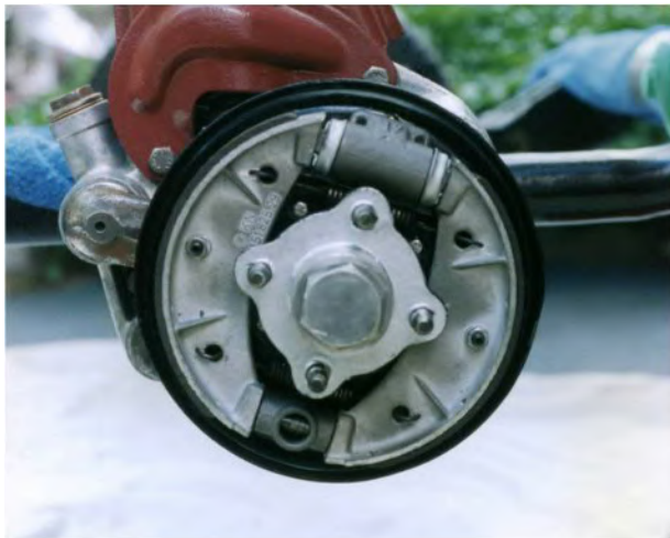
Drum brake shoes and wheel cylinder on backing plate (drum removed)
