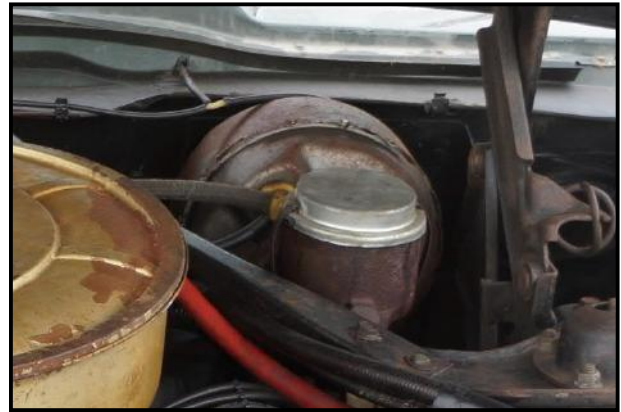
Single-circuit master cylinder, integral reservoir, metal cap
