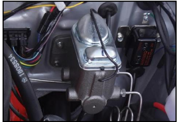
Dual-circuit master cylinder, integral reservoir, metal cap
