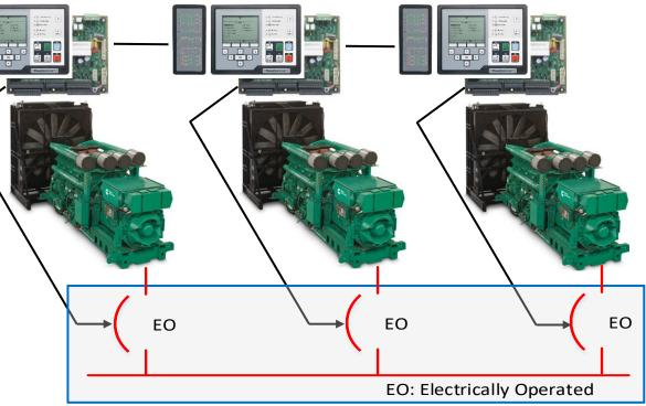
Common point of power connection such as a switchgear or a switchboard
