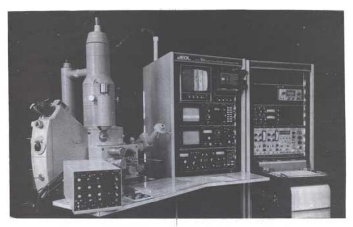
Scanning electron microscope/electron microprobe analyser used for examination and chemical analysis of minute areas of solid surfaces down to 2-3 microns in diameter. This photo illustrates the complexity and (Photo: 11R5) sophistication of modern analytical equipment.
