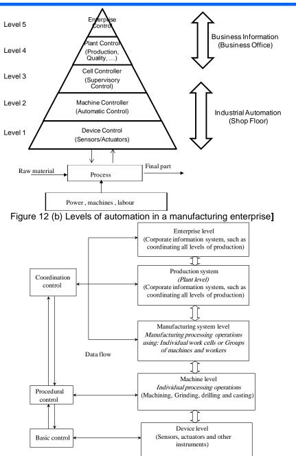
Figure 12(c) Control levels into the levels of automation in manufacturing enterprise
