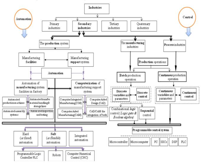
Figure 12(a) Production, Manufacturing control and automation in production system.
