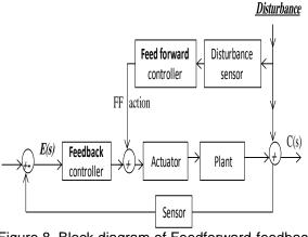
Figure 8 Block diagram of Feedforward-feedback control algorithm
