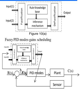
Figure 10(b) example of fuzzy logic algorithm expansion to fuzzy-PD, fuzzy-PI, fuzzy-adaptive algorithms
