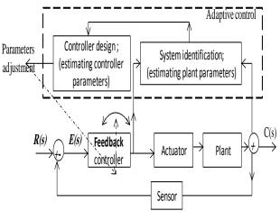
Figure 9 Adaptive control algorithm
