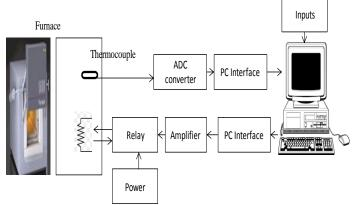
Figure 6 an example of temperature, computer based control system, of an eclectic furnace [25].
