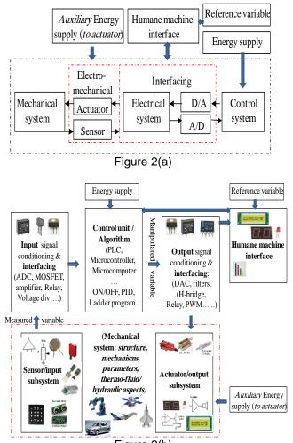
Figure 2(b) Figure 2(a)(b) Working principle and main subsystems of Mechatronic products
