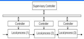
Figure 12 (e) Distributed computer control using local controllers[15][40-42]
