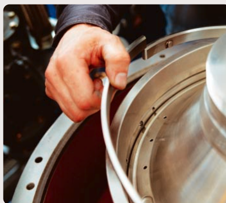
CentriLock lifts out and snaps in easily – without any threads to wear.
