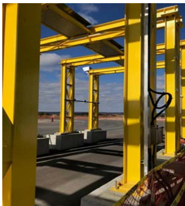
Figure 9. Nuclear Material Transfer Monitor equipped with neutron slab detector
