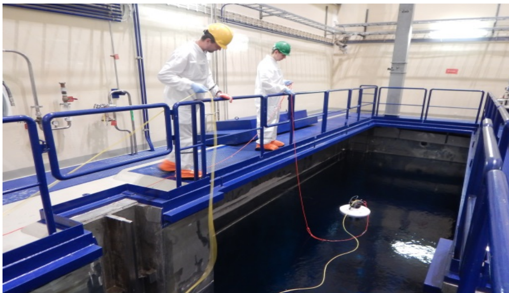
Figure 10. Field test of the USV platform, supporting the verification of spent fuel
