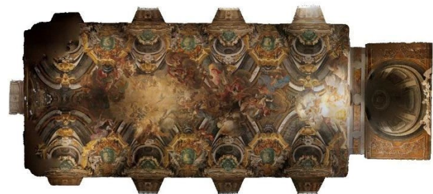
Figure 8. Orthogonal projection of the geometry of the vault and the paintings that decorate it
