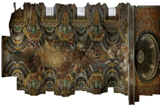
Figure 9. Cylindrical projection of the geometry of the vault and the paintings that decorate it
