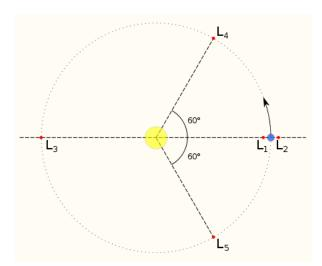
FIGURE 3. The locations of the Lagrange points (image from Wikipedia [10]).
