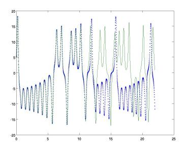
FIGURE 14. A graph of x vs. t, with r = 28. The dotted line corresponds to an initial position of (5,5,5) while the solid line corresponds to an initial position of (5.01, 5, 5) (image created in MATLAB).
