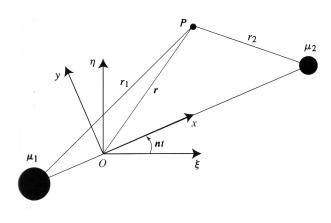
FIGURE 1. The three-body problem: two masses and a particle. Note that the z axis and the  $\zeta$  axis are out of the page (from Murray & Dermott [6]).
