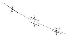
FIGURE 12. The slopes used in the RK4 method (image from Press et al. [7]).
