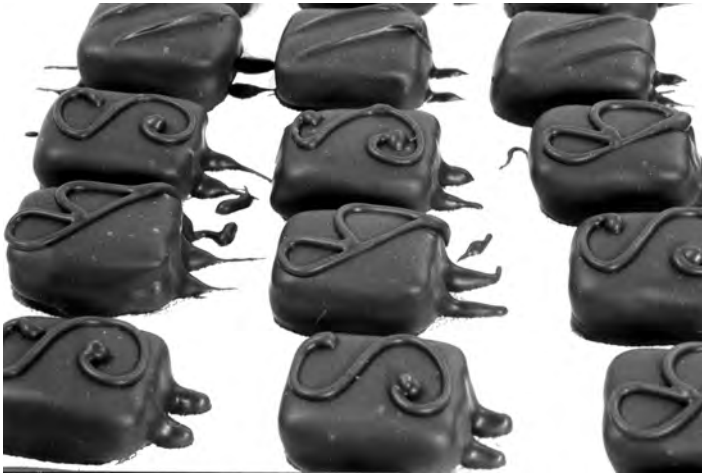
Figure 7.15 Chocolate with “tails” on a cooling tunnel belt.
