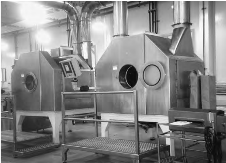
Figure 7.18 Rotating drums used for chocolate or sugar coating.
