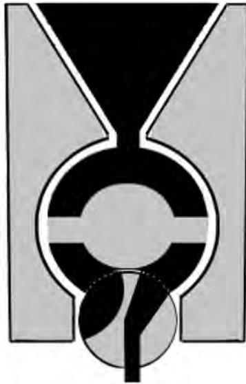
Figure 7.5 Diagram of piston-type depositor to put a measured amount of chocolate into a mould.
