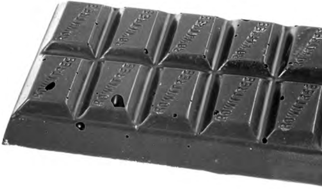
Figure 7.6 Holes in chocolate caused by air bubbles.
