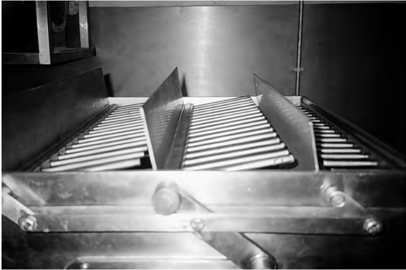
Figure 4.17 Louvres on top of a Frisse conche.
