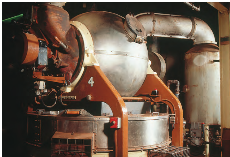
Figure 3.1 Ball roaster for cocoa beans.
