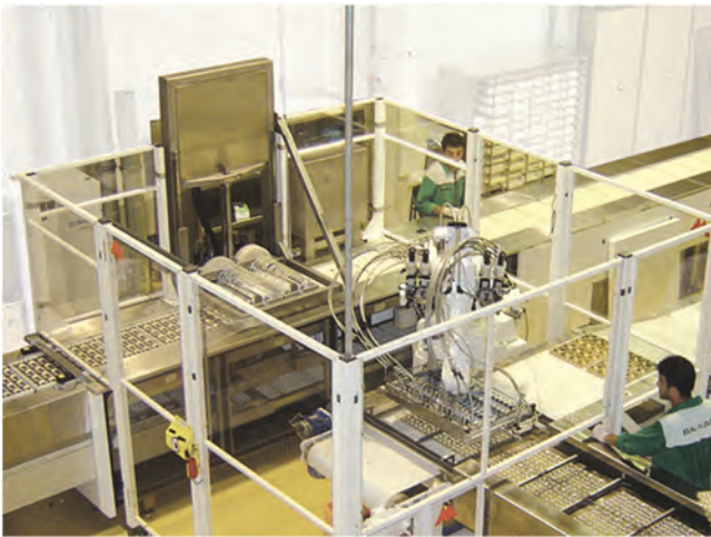
Figure 10.7 Robots packing boxes of chocolates. (Aasted.Mikroverk ApS Denmark).
