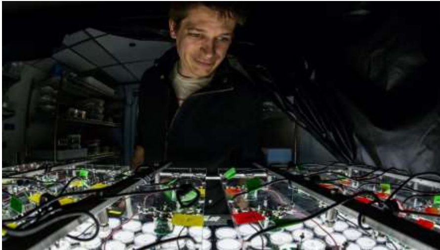
Daniel Kronauer looks over one of his ant tracking systems. Labeled ants are placed in the white dishes and tracked via webcams.
