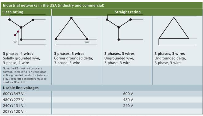
Y describes the solidly grounded circuit. The value "Y" indicates the voltage between the phases (e.g. 480 V), and the value behind the slash indicates the voltage between the phase and the grounding or the neutral conductor (e.g. 277 V with 480 V voltage between the phases).
