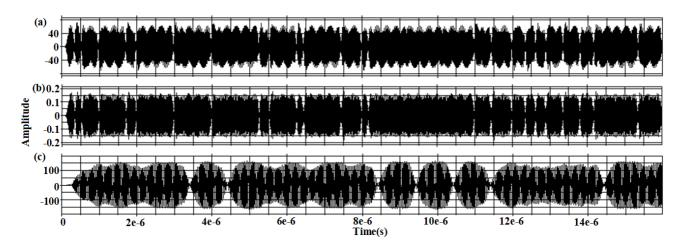
Fig. 5 The export wave: (a) of transmitter; (b) after once frequency conversion; and (c) after twice frequency conversion. Note that (a), (b) and (c) have the same horizontal axis.
