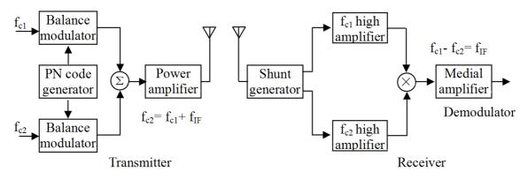
Fig. 1 Theoretical roadmap of the direct sequence spread spectrum
