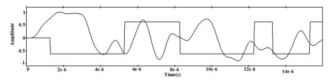
Fig. 6 The export signals add with original signals after Coatas loop demodulation
