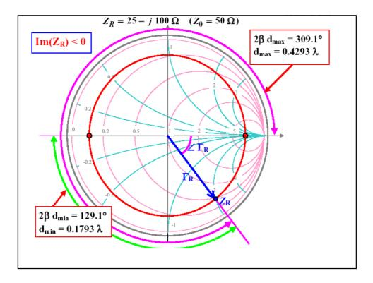
Given  $\Gamma_R$  and  $Z_R \Rightarrow$  Find the Voltage Standing Wave Ratio (VSWR)
