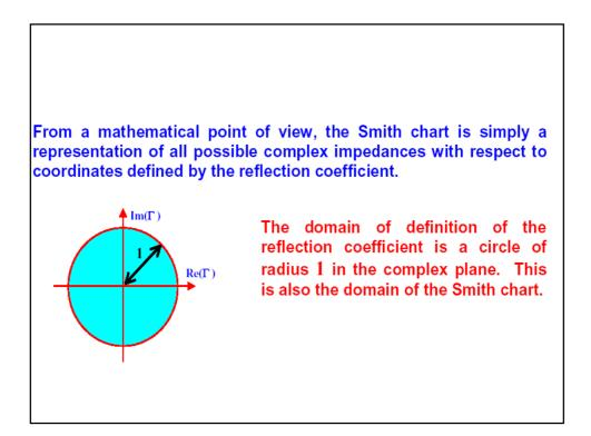
The goal of the Smith chart is to identify all possible impedances on the domain of existence of the reflection coefficient. To do so, we start from the general definition of line impedance (which is equally applicable to the load impedance)
