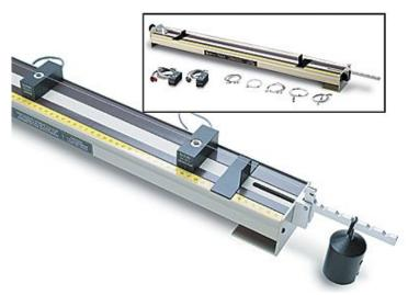
The Pasco sonometer showing weights sound sensor and driver.
