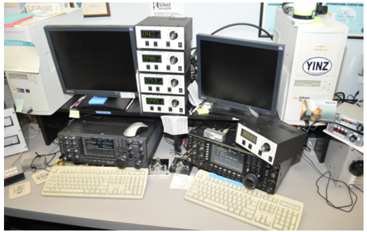
One of the operating positions, featuring a pair of Icom transceivers. (Photo by Mark Haverstock K8MSH)
