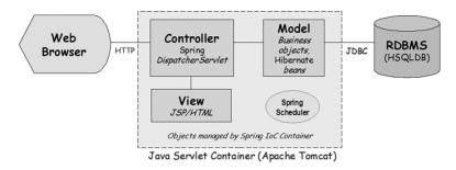
Figure 7.1 High-level architecture diagram for Time Expression.
