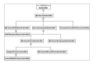
Figure 7.3 Class diagram showing a partial list of Spring controllers.
