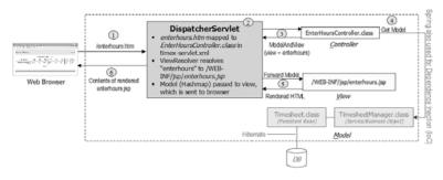
Figure 7.2 End-to-end flow for Enter Hours screen using Spring and Hibernate.
