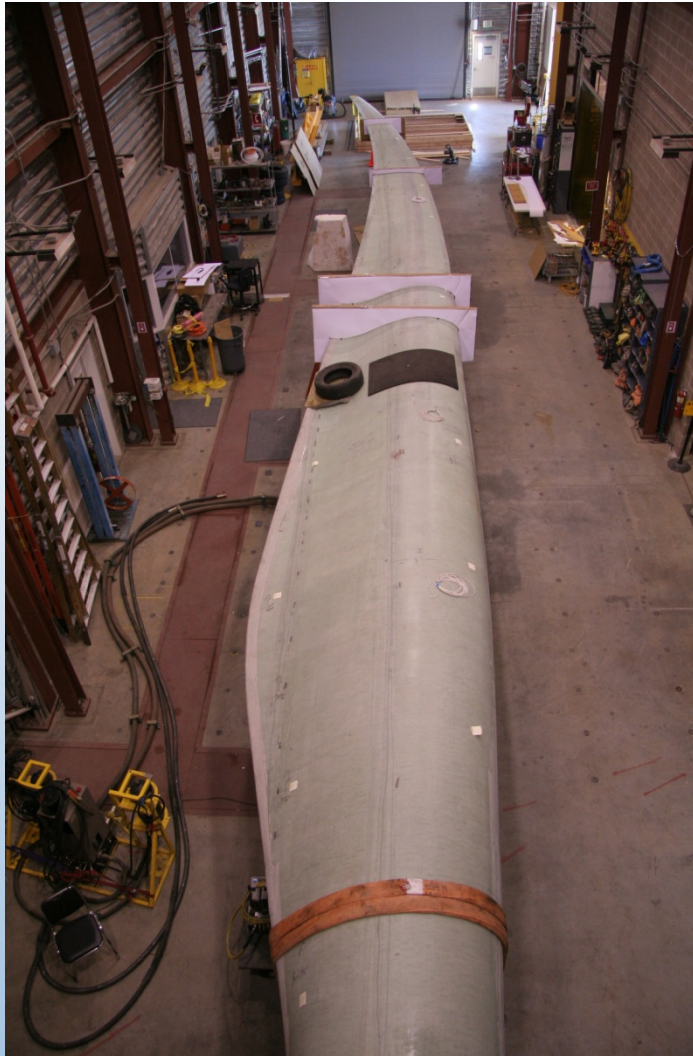
Structural Test of Knight and Carver Blade Test preparation of a swept blade providing twist-flap coupling for gust load reduction
