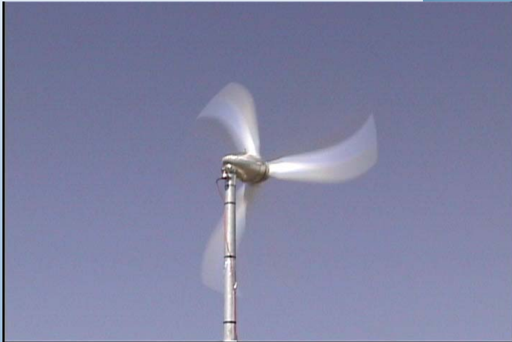
Southwest Windpower Storm 1.8 kW Wind Turbine, 3.7 m diameter
