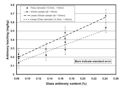
Figure 10. The relationship between composition and leaching. Average results of Sb leaching tests (EN 12547-4) on rolled plate glass for Photovoltaic panel cover. ICG TC13 document, 2010.
