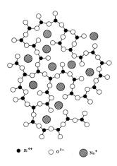
Figure 6. Glass structure showing the silicon tetrahedrons linked together to form the network. Larger ions such as  $Na^+$  are placed outside the tetrahedron. Zarzycki, 1982.
