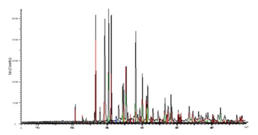
Figure 4. X-Ray Diffraction pattern of a mixture of sand (quartz), soda ash, limestone and dolomite. Horizontal axis: 29, vertical axis: intensity (counts).
