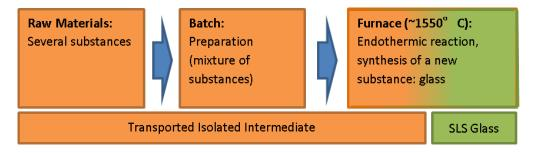
Figure 2. Formation of the substance SLS Glass from raw materials.
