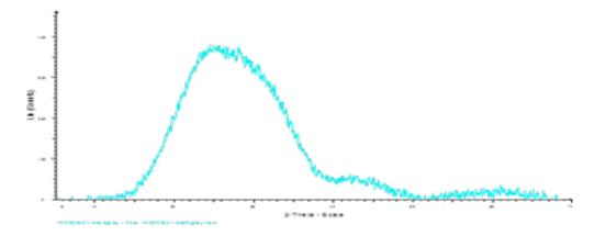
Figure 5. X-Ray Diffraction pattern of soda lime silicate glass. Due to the amorphous glass structure of the substance, no X-ray diffraction peaks appear. Horizontal axis: 29, vertical axis: intensity (counts).
