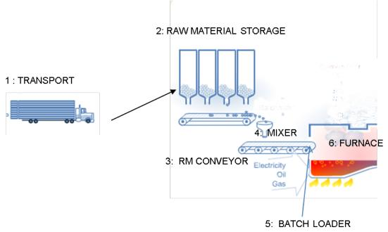
Figure 1. Raw material preparation and feeding to the furnace for the making of SLS glass.
