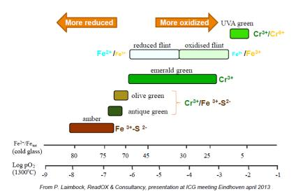
Figure 9. Effect of the redox state of the glass on its colour. Redox vs. colour of Fe & Cr-containing glasses. Hubert, 2015.
