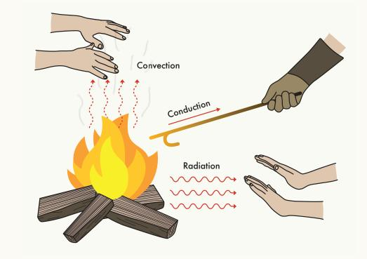
Figure 1. Three types of heat transfer: convection, conduction, and radiation.
