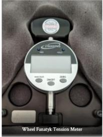
The Centrimaster tool is a high precision analogue tool from Germany which I have found to be incredibly accurate, and the Wheel Fanatyk tension meter is an industry classic, based on an original design from Jobst Brandt (engineer and author of the definitive book "The Bicycle Wheel"). Both are calibrated and supplied with reliable charts of the readings for different spokes,
