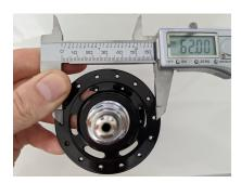
Manufacturer supplied - checked with Vernier callipers for unknown / new hubs (where dimensions are not available).
