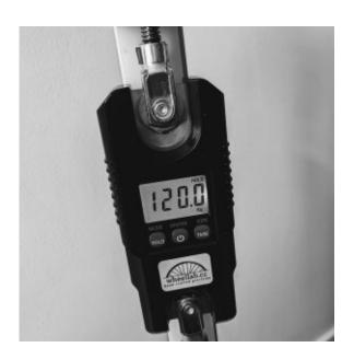
I use a custom built Tension Calibration device from GRS Engineering, who specialise in high end tooling for bicycle wheel building. This allows me to put a calibrated known load on spoke samples, and then measure what the reading will be on a spoke tension meter for that tension.
