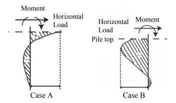
Figure 1 Bending moment distribution in a pile
