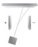
The deflected beam is alpha radiation because it is deflected toward the negatively charged plate. The undeflected beam must be neutral  $\gamma$  gamma radiation.
