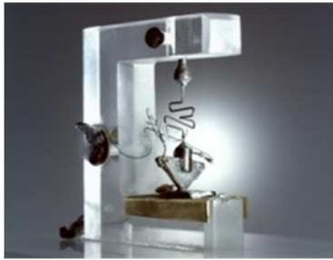
Figure 9: The Shockley transistor—the first transistor.
