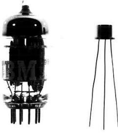
Figure 6: Vacuum tube, single transistor, and chip transistor (the dot) [IBM, 1964].
