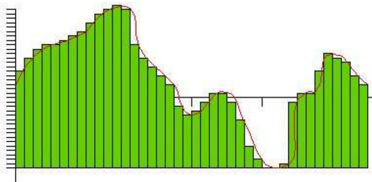
Figure 15: A sound wave and the samples of that sound wave (green bar height) over time
