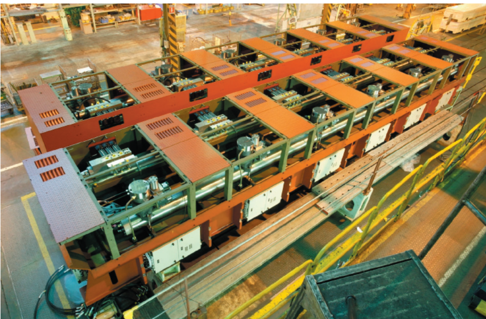
Fig. 10 below: The two sections of rail unit for a 12-cylinder RT-flex96C engine during the course of assembly. [04#076]
