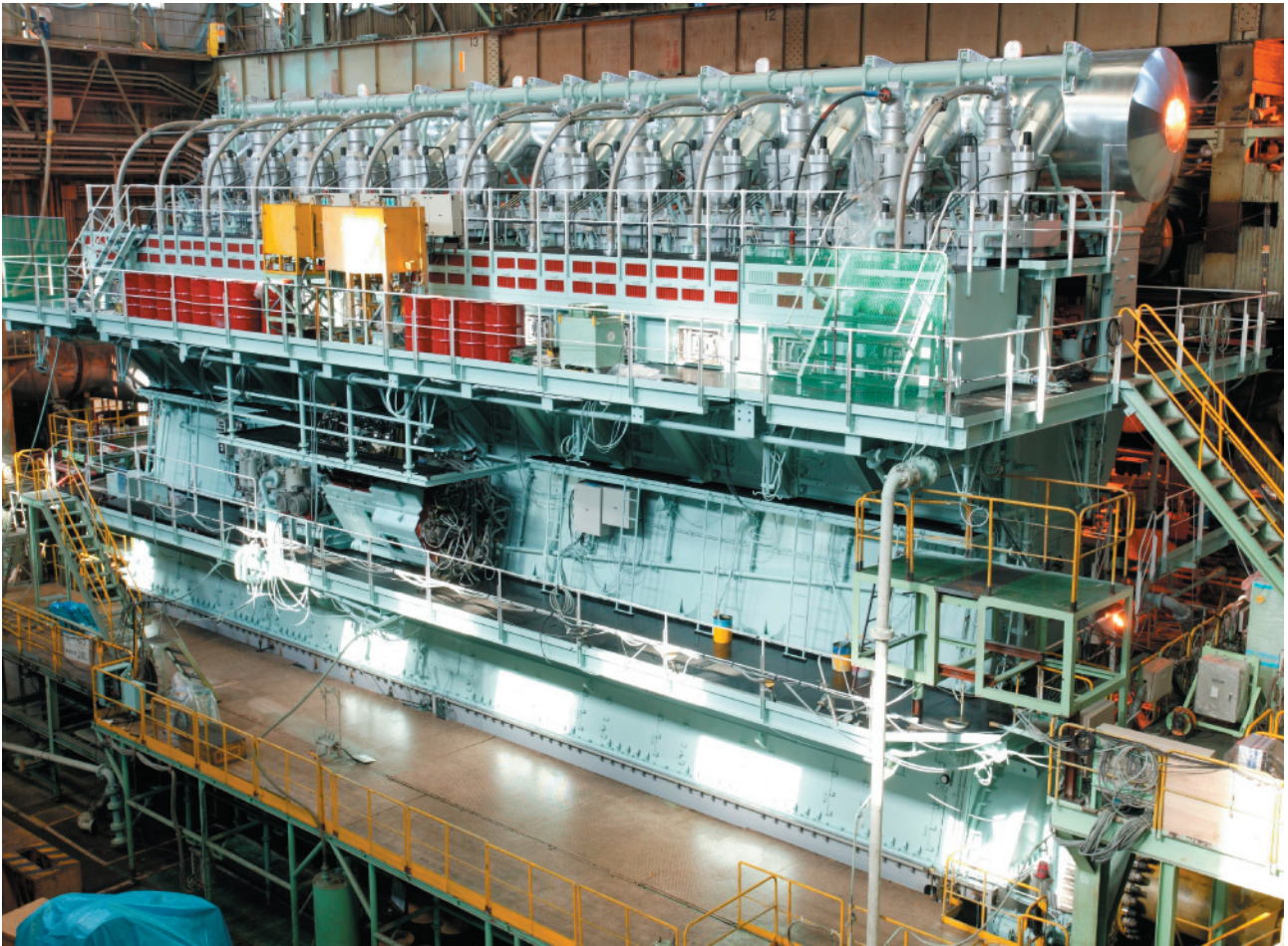
Fig. 21: The world's most powerful common-rail engine, the Sulzer 12RT-flex96C engine develops 68,640 kW at 102 rpm, and measures about 24 m long by 13.5 m high. It passed its official shop test in June 2004. The supply unit shown in figure 4 can be seen at the middle of the engine.
