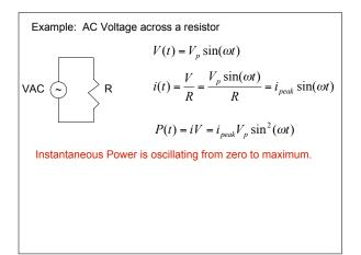
We might be interested in the average (over time) power delivered to the resistor.  $P(t) = iV = i_{peak}V_{peak}\sin^{2}(\omega t)$  $< P(t) >= i_{peak}V_{peak} < \sin^{2}(\omega t) >= \frac{1}{2}i_{peak}V_{peak}$  $< P(t) >= \left(\frac{1}{\sqrt{2}}i_{peak}\right)\left(\frac{1}{\sqrt{2}}V_{peak}\right)$  $P_{ave} = i_{rms}V_{rms}$ Same form as before, but now RMS values.
