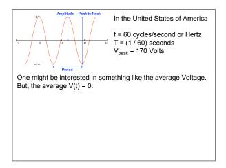
$V_{rms} = V(\text{root mean square}) = \sqrt{\langle V_{\gamma}^2 \rangle}$ Time Average of Voltage squared.  $V_{rms} = V_p \sqrt{\langle \sin^2(\omega t) \rangle} = V_p \sqrt{1/2} = V_p / \sqrt{2}$ Time Average of sin<sup>2</sup> or cos<sup>2</sup> over many cycles = 1/2  $V_{rms} = 170V / \sqrt{2} = 120 \text{ Volts}$ This is how we refer to the US Standard Voltage.
