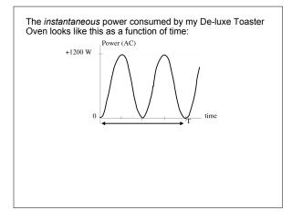
1200 W -Which of the following is correct? <u>V rms</u> <u>I rms</u> 120 V 10 A (=1200/120) P ave <u>A</u>: 1200 W 7 A (=1200/170) <u>B</u>: 1200 W 170 V <u>C</u>: 600 W 120 V 5 A (= 600/120) <u>D</u>: 600 W 170 V 3.5 A (=600/170)  $\underline{E}$ : None of the above is right.
