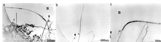
Fig. 17 Bending of \text{Si}_3\text{N}_4 nanowire: (a) bend to right, (b) at original position when the average density of the electron beam is small, and (c) bend to left. The B is marked as the center of the illumination beam (ref. 103).
