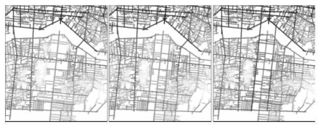
Figure 10: Axial analysis of the Chaharbaghe-Bala area: left: existing; centre: the area with the two proposed streets; right: the area with the two proposed streets extended to the north of the river
