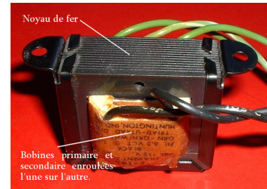
Figure 3.23: A real-life transformer. The wire of the primary is black, those of the secondary are green (the middle wire is the ground wire). [Photograph : Wikipedia]
