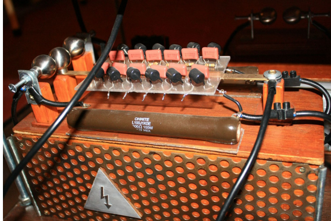
Figure 4.38: The protection filter assembled. The NST is in the wooden box just under the filter.
