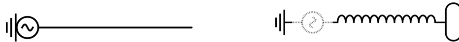
Figure 3.28: Analogy between a quarter-wave antenna and the secondary circuit of a Tesla coil.
