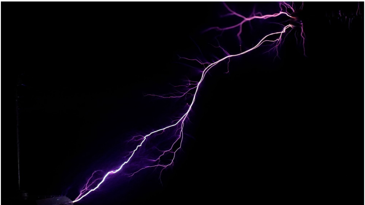
Figure 4.3: A 40 cm spark (looks like a natural one!). 1/30s shutter speed. [Photograph: Jean-Louis Colot]
