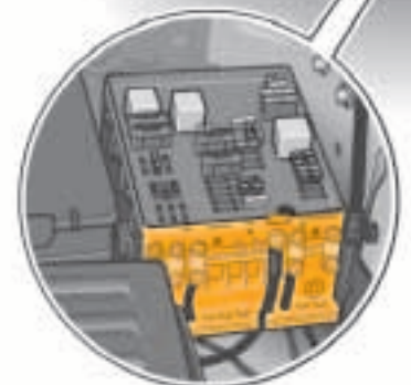
Back-up fuse box on left in engine compartment
