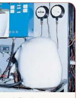
"Snowball" underwent a continuous flood-back test in the Trane compressor life test facility for 27 years, before finally ceasing to operate in 2000. The test demonstrates the reliability of the compressor under conditions like low indoor airflow or system overcharge.
