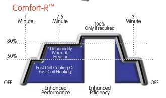
Comfort-R<sup>™</sup> provides improved dehumidification in cooling start up and warmer air start up in heating. This is accomplished by running the fan at a slower speed during start up. A simple change of the blower control setting provides this enhanced level of comfort.
