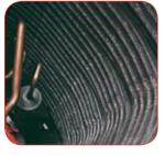
Spine Fin<sup>™</sup> coils are fabricated in continuous lengths. Because of the number of leading edges, one row has the ability to transfer the same amount of heat as three rows of plate fin.
